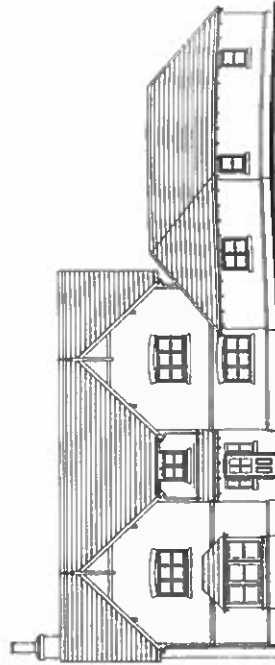
HOUSE TYPE H - FRONT ELEVATION SCALE 1:200
